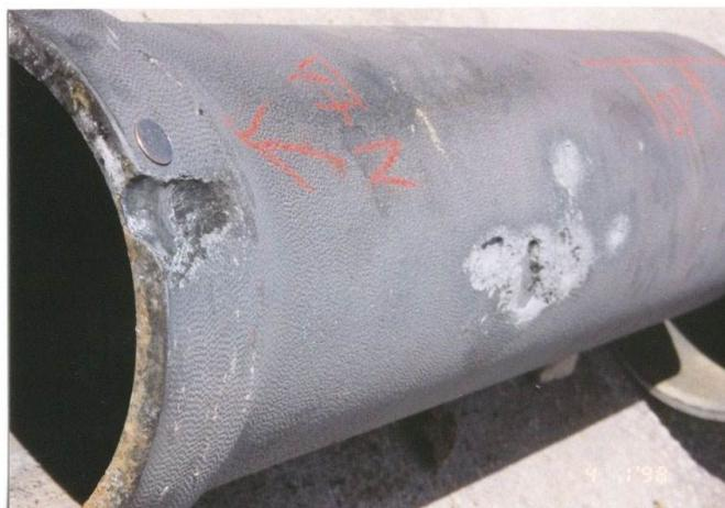
Fig-1: typical corrosion cells in cast-iron pipe
